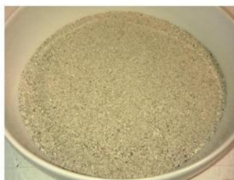
Fine mussel shell sand, FMS (heat treatment, crush and sieve)
