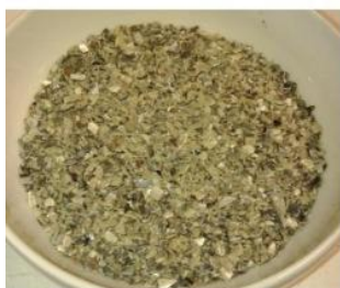
Coarse mussel shell sand, CMS (heat treatment, crush and sieve) FIGURE 4. Mussel shell
