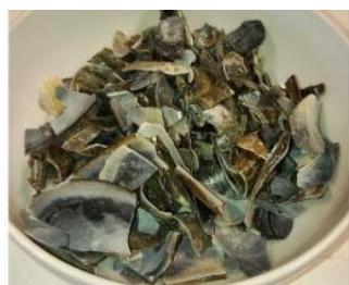
Mussel Shell gravel, MG (heat treatment)
